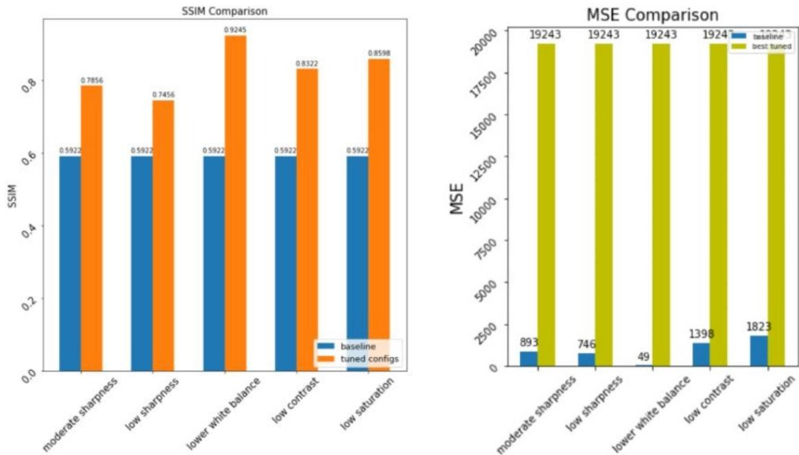
Figure 13: Top Configurations SSIM and MSE
